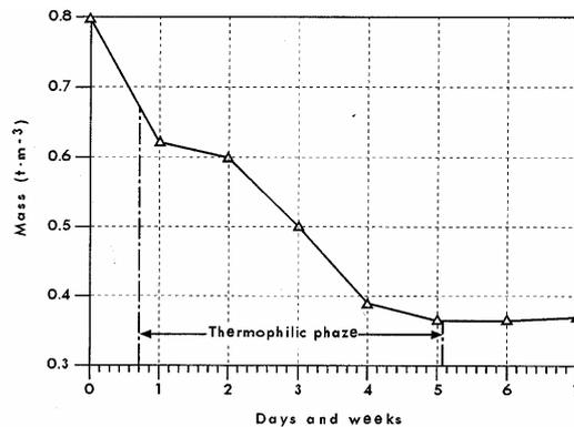
Figure 2. Depository weight changes during crude solid manure aerobic care
