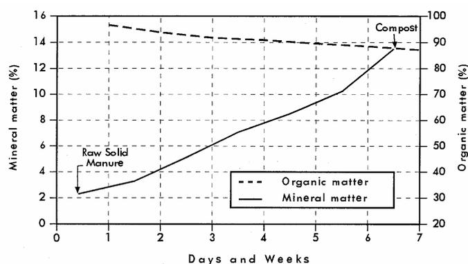
Figure 4. Mineral and organic matter content changes in the depository during solid manure aerobic care
