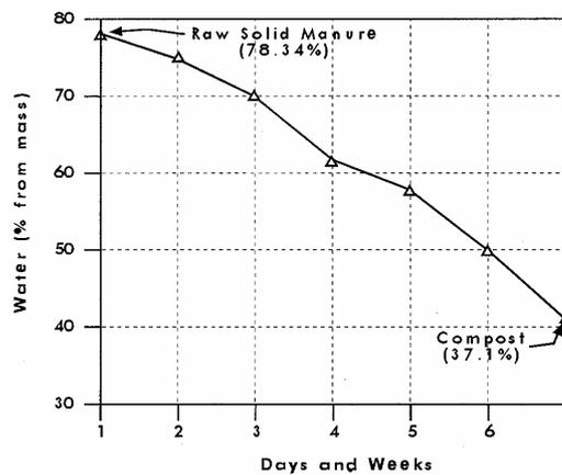
Figure 3. Water content changes in depositories during solid manure aerobic care
