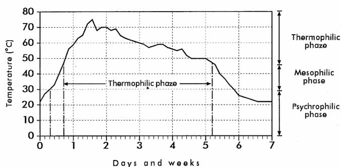
Figure 1. Temperature changes in depositories during crude solid manure aerobic care
