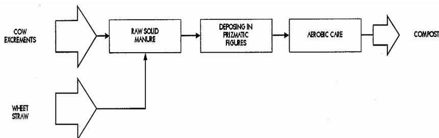
Scheme 1. Technological procedure of the experiment
