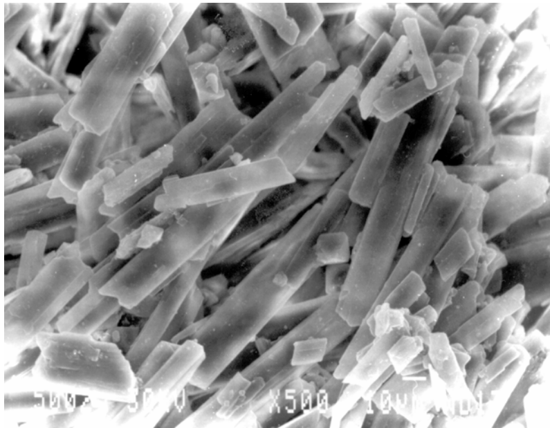
Fig. 5. SEM micrograph of crystalline structure of phosphogypsum precipitate (×500)
