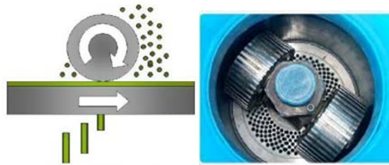
Figure 2: The working principle of pellets machine with a flat matrix
