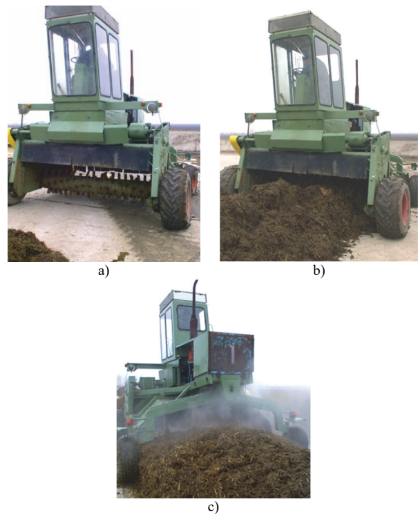
Figure 1 The self-propelled machine Kompomat 1: (a) prototype view; (b) untreated (raw) pile; (c) machine in work pile treatment
