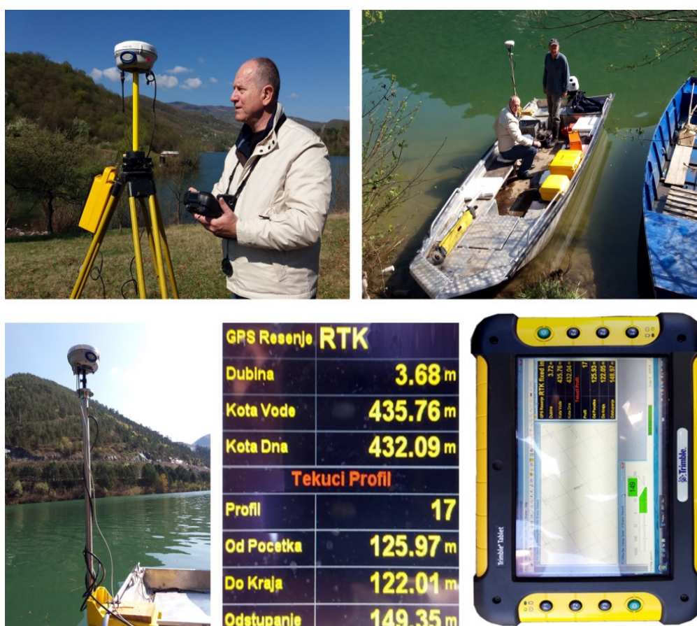
Figure 17. Bathymetric survey of the Potpec reservoir and detail of the equipment used.
