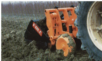
Slika 7. Rad rotacionog ašova na teškom i raskvašenom terenu, [24] Figure 7. Operation of the rotary shaft on difficult and task-based terrain, [24]
