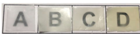
Figure 2. Contact transparency image of the plain poly( \epsilon -caprolactone) PCL film (A) and the PCL-based films containing: 5% (B), 10% (C), and 20% (D) SE.
