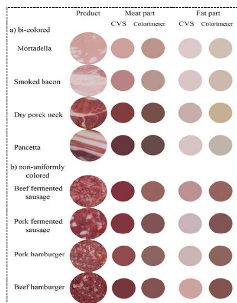
Figure 4. Color of bi and non-uniformly colored meat products as measured by the two methods [2]
