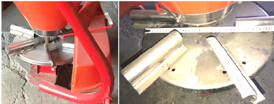
Figure 1. A centrifugal fertilizer spreader, having a flat disc with straight radial vanes.
