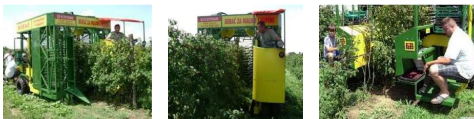
Slika 4. Samohodni mehanički berač maline i kupine firme "ELEKTRONIK" [4] Figure 4. Self-propelled Mechanical Berry Harvester made by "ELEKTRONIK" [4]
