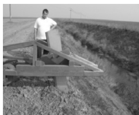
Figure 7. Drainage plough in working.
