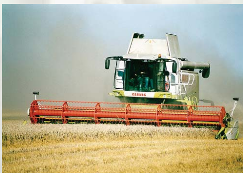
Sl.5. Izgled i položaj laserskog sistema Laser pilot na kombajnu Lexion 580 [6] Fig.5. The appearance and position of the laser system on combines Lexion 580 [6]
