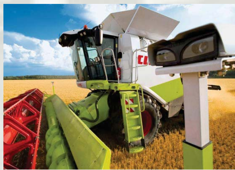
Sl.5. Izgled i položaj laserskog sistema Laser pilot na kombajnu Lexion 580 [6] Fig.5. The appearance and position of the laser system on combines Lexion 580 [6]
