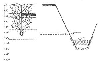
Fig. 8. - The scheme of mole's drainage
