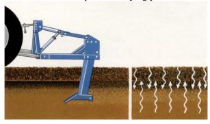
Fig. 3. - Example of subsoiler's work – ascending and descending moves of water through soil layers
