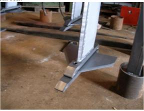
Fig. 9. - Working units of vibrating subsoiler VR-5(7)
