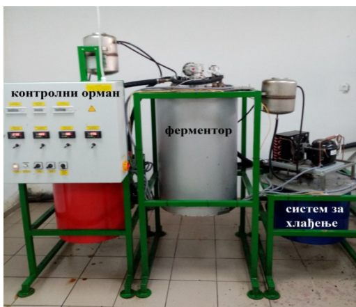
Figure 1. Fermenter used for fermentation of apple juice (location: Laboratory for Unit Operation and Biochemical Engineering; Faculty of Agronomy, Čačak)
