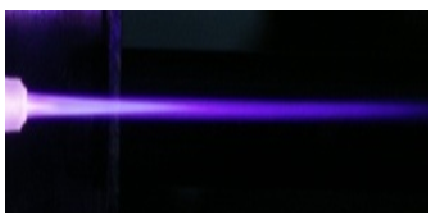
Figure 1: Helium atmospheric plasma in ambient air at the end of the tube
