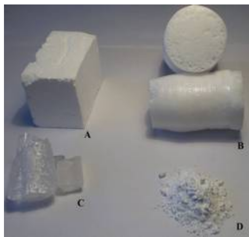
Fig.1 Samples of aluminum oxide: A- densified sinter as brick, B- fused aluminum oxide as rods, C- Verneuil sapphire, D- nanopowder
