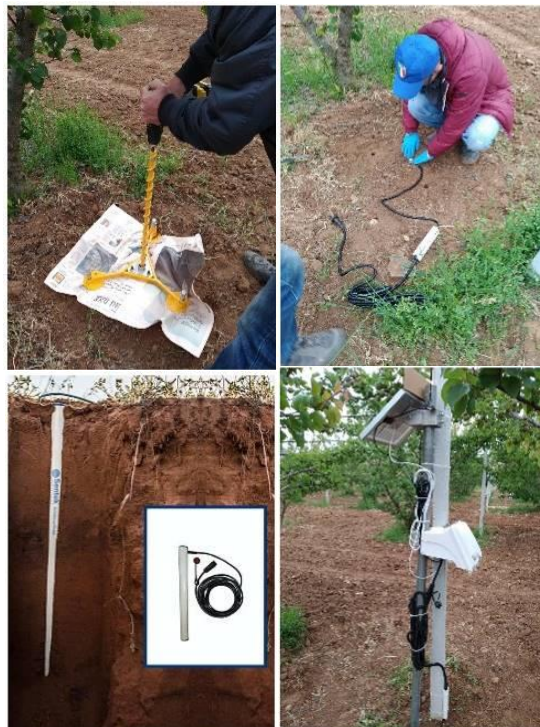
Figure 1. Drill&Drop automated sensors installed in an Apricot farm, Southern Italy.
