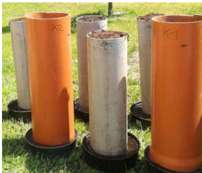
Figure 4. Capillary saturation to 50°hPa.
