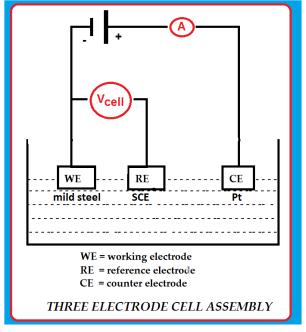
Figure 1. Circuit diagram of three-electrode cell assembly
