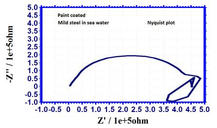
Figure 9. Nyquist plot of paint coated mild steel in seawater Slika 9. Nyquist-ova kriva mekog čelika premazanog bojom u morskoj vodi
