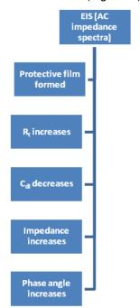
Figure 5. Correlation among corrosion parameters of AC impedance spectra
