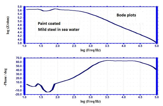
Figure 10. Bode plot of paint coated mild steel in seawater Slika 10. Bode-ova kriva za meki čelik premazan bojom u morskoj vodi
