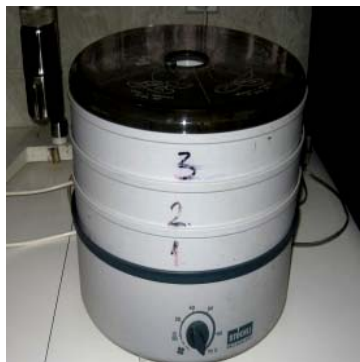
Figure 1. Laboratory dehydrator Stöckli, Switzerland with three mesh trays.
